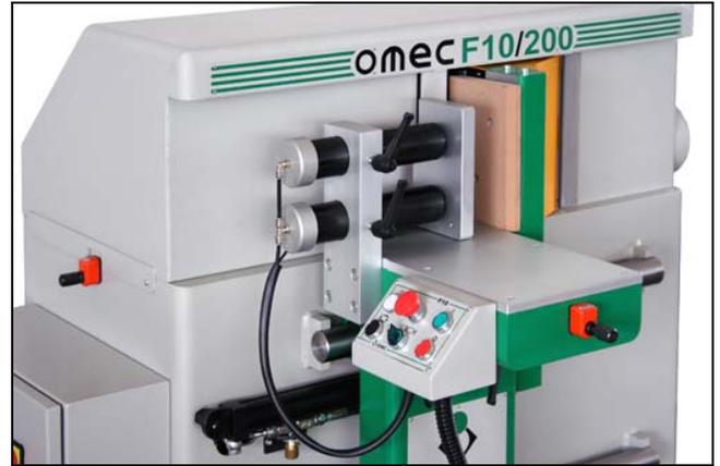
The bigger model, F10/450, can machine bundles of boards of a max. height of 450mm. Both models perform a cutting cycle every six seconds.
