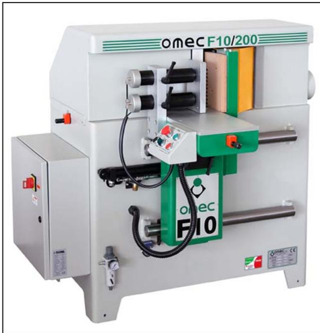
This machine is fitted with a cutter arbor that is suitable for the manufacture of joints of different heights. Pieces are machined in bundles, first on one side and then on the other side, with an automatic feed mode. Each bundle of workpieces is pushed towards the cutter arbor by a cylinder that is driven by a hydraulic station. Bundles are locked with a pneumatic system that is controlled by a valve.
