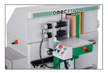
The bigger model, F10/450, can machine bundles of boards of a max. height of 450mm. Both models perform a cutting cycle every six seconds.
