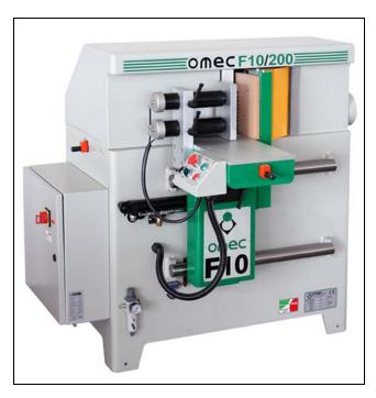
This machine is fitted with a cutter arbor that is suitable for the manufacture of joints of different heights. Pieces are machined in bundles, first on one side and then on the other side, with an automatic feed mode. Each bundle of workpieces is pushed towards the cutter arbor by a cyilinder that is driven by a hydraulic station. Bundles are locked with a pneumatic system that is controlled by a valve.
