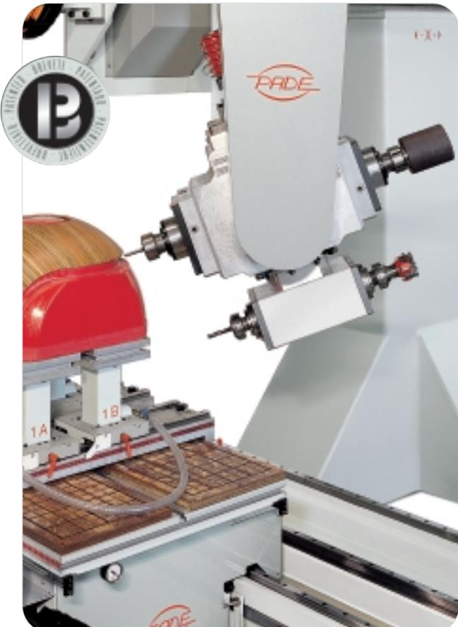
**T**his head comprises 4 motors of which 3 aligned in cross formation and 1 horizontal with two exits. The main advantages of this solution are: 5 available spindles; possibility to execute operations ‘flush’ to the machine fixing; Execution of operations in extremely tight spaces; Machining components with M4
