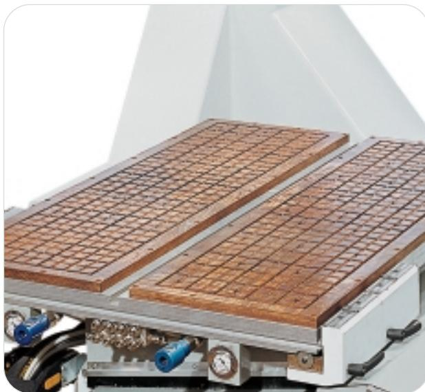
**W**orking tables made of rexilon for the vacuum clamping of pieces. The surface is shaped for using the rubber gasket which delimits the vacuum used area.
