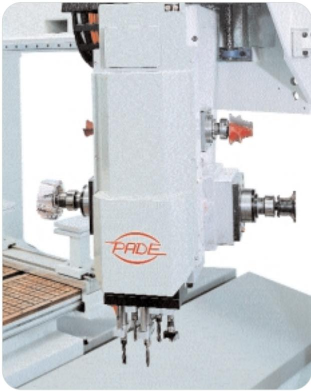
Independent boring unit with 5 spindles, 32 mm centres, located on the sliding guide with 360° swivel around C axis. A dedicated software (optional) will automatically optimise the sequence and selection of the operating spindles in accordance with the hole settings and boring distances.
