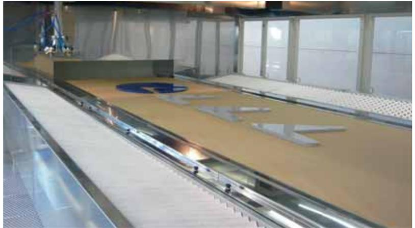
3D scanner (option) makes it possible for example the selective spraying of mouldings and grooves and makes the machine perfect for applications such as glue spraying on work-pieces for membrane-pressing or such as the application of antique effect stain.
